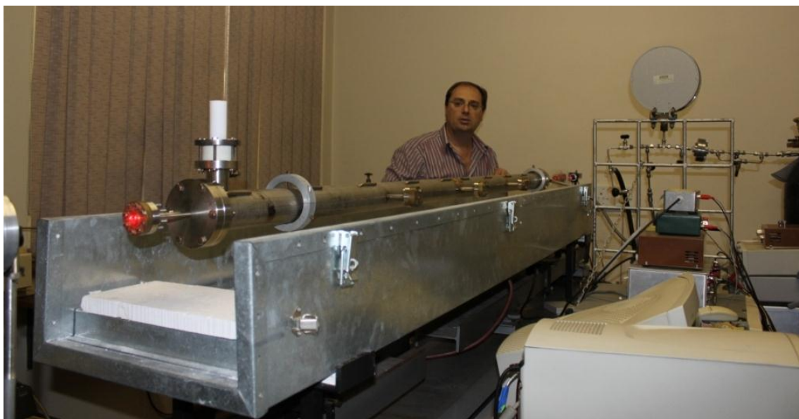
Picture Caption: The Buckingham-effect experiment, used to measure molecular electric quadrupole moments
